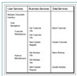
Figure 1.5 An application broken into three tiers of services.
