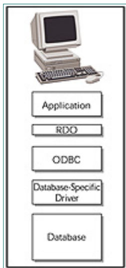
Figure 4.4 The Remote Data Objects model.
